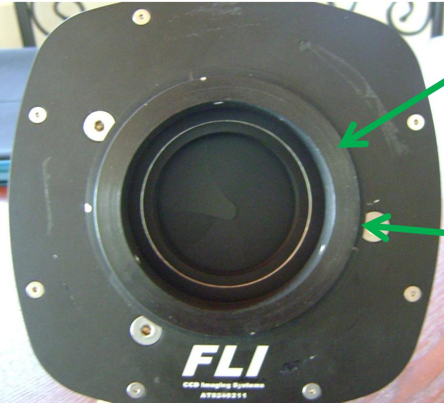
And on this ring to loosen three grub screws
